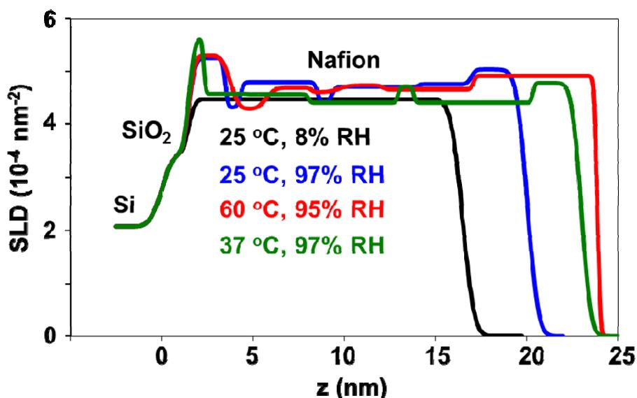
SLD profiles of 150 Å Nafion layer on native SiO<sub>2</sub> as a function of temperature and humidity. Note the large step in the thickness, both between 8 and 97% RH and 25 and 60°C at 97-95% RH.
