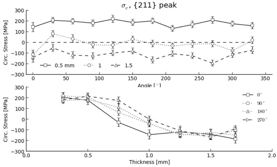
**Figure 2** Residual stress in circumferential direction. Top: as a function of circumferential angle for three depths. Bottom: as a function of thickness for four circumferential locations.
