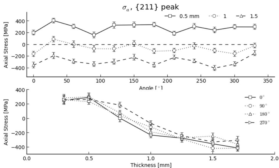
**Figure 1** Residual stress in axial direction. Top: as a function of circumferential angle for three depths. Bottom: as a function of thickness for four circumferential locations.
