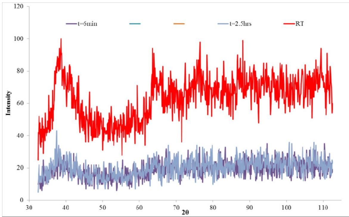
**Figure 2:** Diffraction patterns obtained from the neutron beam during heat treatment experiments of  $\text{FeCo}_{35.2}\text{B}_{4.3}\text{Si}_{2.8}\text{Nb}_{7.7}$  droplets of size 125  $\mu\text{m}$  atomized under nitrogen.
