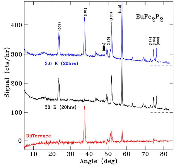
FIG. 1: Powder neutron diffraction patterns for  $\text{EuFe}_2\text{P}_2$  taken at a wavelength of 2.3672(1) Å above (50 K) and below (3.6 K)  $T_C$  showing the development of magnetic scattering on cooling. The intensity changes can be seen more clearly in the difference pattern shown at the bottom of the figure.
