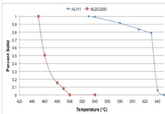
Fig. 2. Fraction solid development of solid Al and Al<sub>2</sub>Cu.
