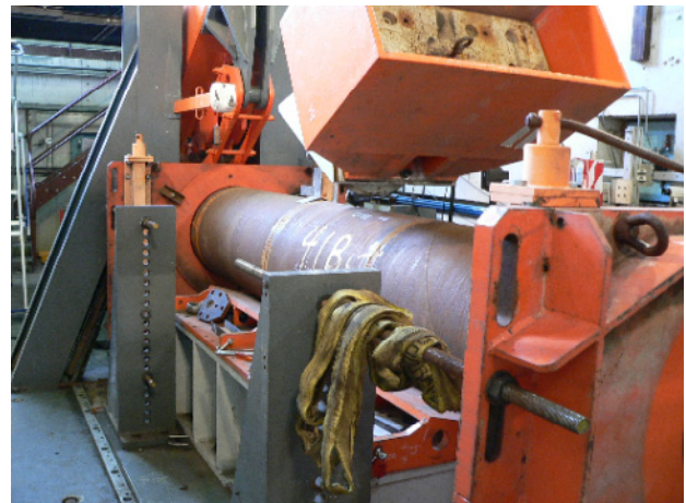
Fig. 1 the PAR (experimental backhoe) setup in the GdF Suez laboratory in St. Denis, France. The PAR is shown in action, creating a gouge in a pressurized pipe. The large orange box is a simulated backhoe bucket, swinging in an arc before impacting the pipe wall at a grazing angle.
