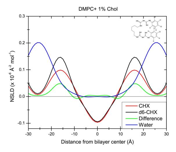
Fig. 1 SLD profile for labeled (black) and unlabeled (red) CHX in a DMPC bilayer doped with 1% cholesterol. The green line is the SLD difference between labeled and unlabeled CHX and the blue line is the water distribution in the sample. The CHX structure (top right) is the most probable orientation as determined by the data and molecular dynamic simulation.
