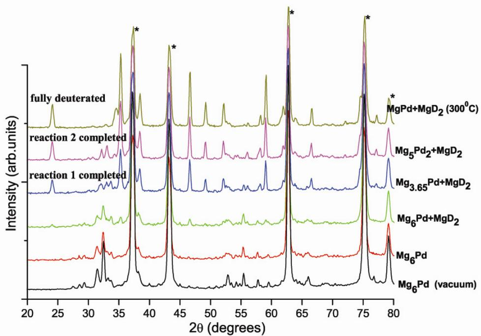
**Fig. 2** Pressure NPD patterns collected during  $\text{Mg}_6\text{Pd}$  hydrogenation. The \* symbol marks the peaks arising from the steel sample holder.
