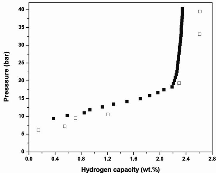
**Fig. 1** Pressure-composition absorption isotherms of activated Mg<sub>6</sub>Pd at 350 °C. The solid symbol are PcT points collected in the laboratory; open symbols are PcT points collected during at the same time with the PND measurements.
