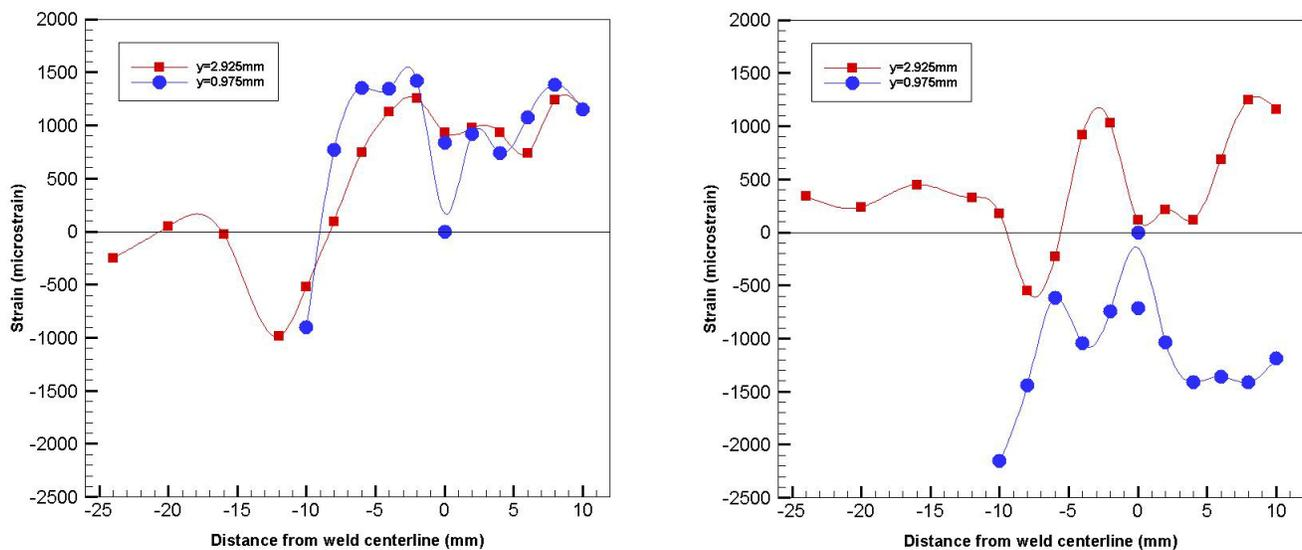
Fig. 1 (left) Longitudinal strain in as-welded plate. (right) Longitudinal strain in hammer peened plate.
