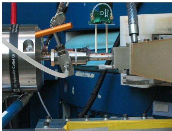
**Fig. 2** In situ biaxial loading experiment at the L3 beamline. (left) Spectrometer, load frame and detector. (right) Close up of a hollow tubular specimen in the load frame grips and connected to the pressurization system.
