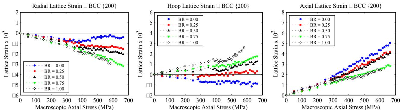
Fig. 5 Lattice strain data for the BCC {200} radial, hoop, and axial fibers at five levels of stress biaxiality.
