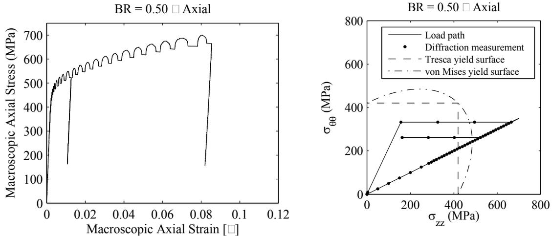
Fig. 3 (left) Representative macroscopic axial stress-strain curve and (right) load path in stress space.
