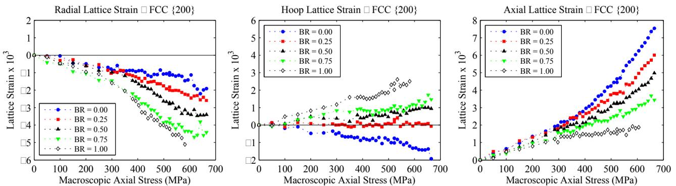
Fig. 4 Lattice strain data for the FCC {200} radial, hoop, and axial fibers at five levels of stress biaxiality.
