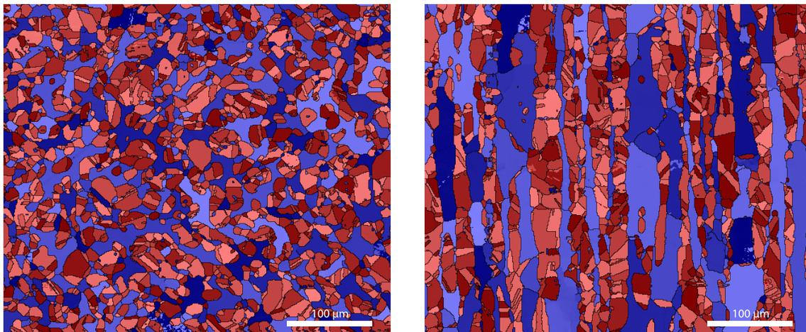
**Fig. 1** Electron backscatter diffraction map of LDX-2101 viewed with the extrusion axis (left) out of the page and (right) vertical in the plane of the page. In these false colored images, austenite is red and ferrite is blue. Grains are shaded according to crystallographic orientation.
