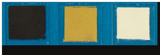
Fig. 1 Comparison of polycrystalline samples belonging to the Sc-V-O system, left: \text{ScVO}_{3.70} , center: \text{ScVO}_{3.94} , right: \text{ScVO}_{4.00}
