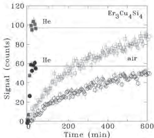
**Fig 2.** Time dependence of two magnetic reflections for samples of  $\text{Er}_3\text{Cu}_4\text{Si}_4$  sealed under helium (solid symbols) and air (open symbols) showing the very different cooling rates. Symbol shapes correspond to those used in Fig. 1. The solid lines show the expected saturation values for the two peaks at 0.34 K.
