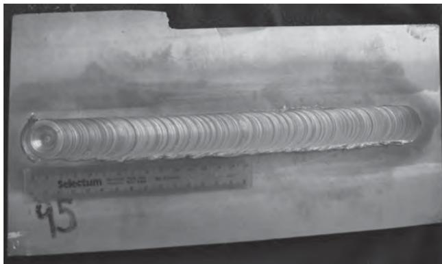
**Fig 1.** NAB cast plate. The FSP volume's top surface features semicircles that correspond to the rotating shoulder. This band of semicircles is surrounded by a blue-tinged region related to the high temperature reached in this region during FSP.
