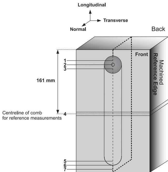
**Fig 3.** Schematic of NAB specimen showing the reference surfaces, coordinate system, and measurement directions.
