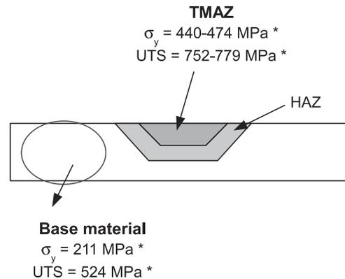
**Fig 2.** Mechanical properties in the TMAZ and in the parent material.
