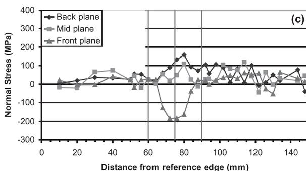
**Fig 4.** Copper {311} stresses for a) the longitudinal, b) the transverse, and c) the normal directions along line 4.
