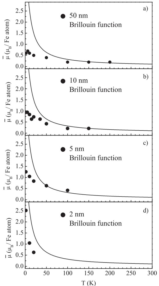
**Fig 1.** Averaged magnetic moment per Fe atom versus temperature of thin  $Au_{97}Fe_3$  films as derived from the fits to the PNR curve (solid circles) compared to a Brillouin function with  $J = 2$  for isolated Fe atoms (solid line).
