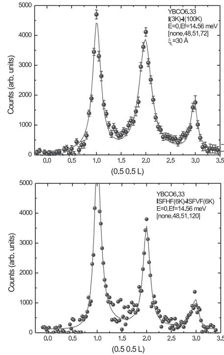
**Fig. 3** Elastic magnetic scattering along the  $(0.5 \ 0.5 \ L)$  obtained from the non-polarized study (top, low temperature minus high temperature background) compared to the polarized data (bottom, low temperature SF vertical field data is subtracted from the horizontal data).
