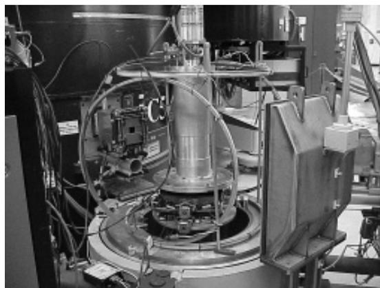
**Fig. 1** Two pairs of coils were used to control the direction of neutron spin at the sample position. The sample is mounted in the closed-cycle refrigerator (centre).
