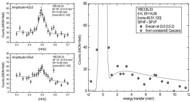
**Fig. 5** Polarized spin-flip inelastic neutron scattering data. Inelastic scans along [HHZ] direction (left) show that the spin directions are isotropic since the HF intensity is twice that for VF. (right) The magnetic spectrum along [1,-1,0] measured by subtracting the VF from the HF data. The spectrum is fitted to a central mode and a modified Lorentzian (right line in the right panel).
