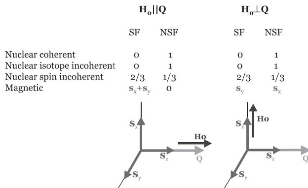
**Fig. 2** Two configurations of the neutron spin at the sample position are shown. For each orientation, the contributions from nuclear and magnetic scattering are listed for both the spin-flip (SF) and non-spin-flip (NSF) components. The spin scattering cross-section  $S^{\alpha\alpha}$  is denoted  $s_\alpha$ .
