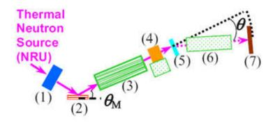
Schematic of the N5-SANS adapted from a tripleaxis spectrometer to an instrument capable of SANS measurements. The components are as follows: (1) sapphire or Be filter. (2) Monochromator. (3) 23-channel CSC. (4) PG filter/21.6 cm long HSC/open. (5) Sample. (6) 48 cm long HSC. (7) 32-wire position sensitive detector.
